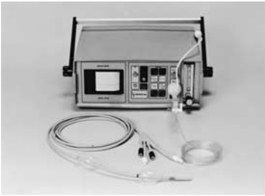
Fig. 1 Measuring devices of SIPS : UROLABMICRO (1151M)™ (Life-Tech Co., Ltd. USA) and Cliny double balloon ileus tube (Create Medic Co., Ltd.).
